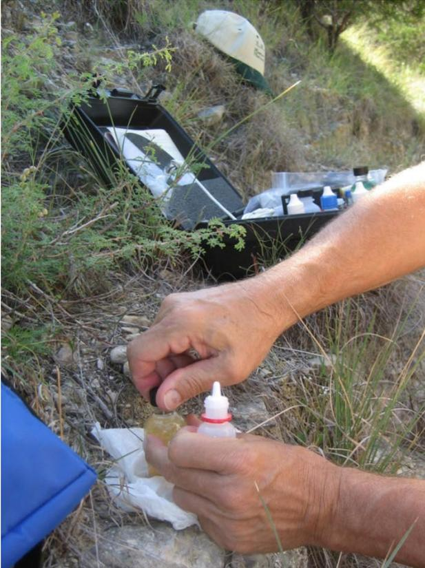
*Preparing a water sample for the dissolved oxygen measurement.*
